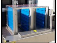
**Estimated Capacity:** 3 Arms re-plugging 7,560 plugs per hour 5 Arms re-plugging 11,160 plugs per hour Power: 230VAC, 3 Phs., 25 A
