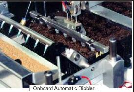
A vacuum is applied to an array of interchangeable syringe needles to accurately pickup and deposit seed in each individual cell.
